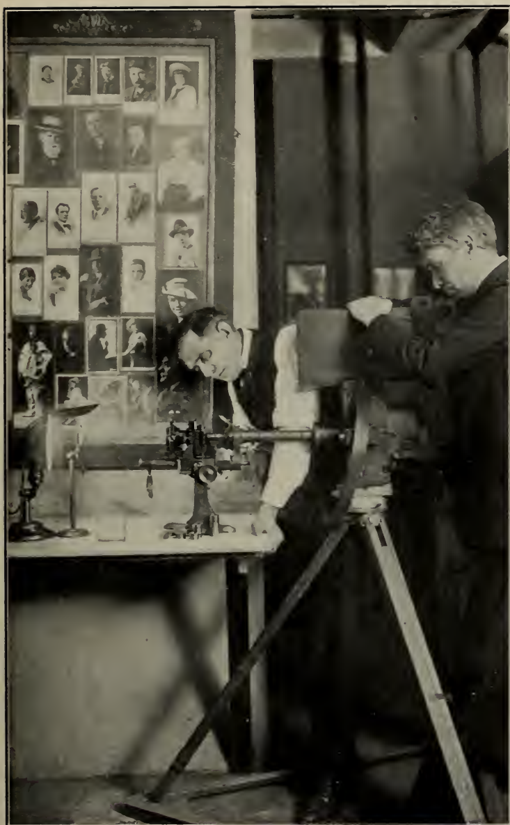
Making a Micro-cinematograph of Bacteria to illustrate a Biological subject at the N. Y. Institute of Photography.
